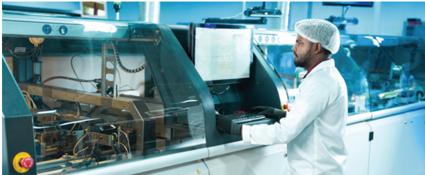
Automated Through-Hole Technology (THT) selective soldering process to ensure fast and accurate assembling process.
