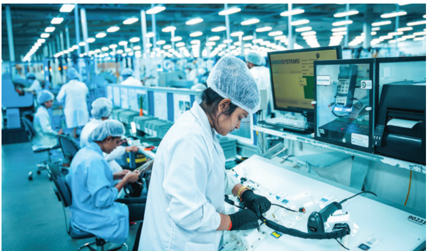
Connectivity test, part of wire harness testing process.
